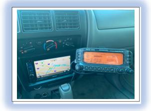
Kenwood 710G Mobile Radio Mounted to a Pana Vise. The Brain of the radio is installed under the driver's seat. The nice part is that I can easily remove the face plate with a press of a button and store it when necessary.
