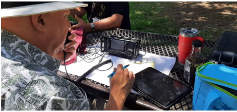
Joe, AK6MB was on his ICOM IC-705 and a Buddipole-mini antenna, making FT8 contacts in Arizona and Texas on 15m.
